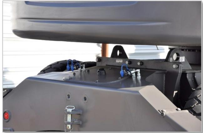
*Valve socket for brake, tip and spread, as well as trailer*
