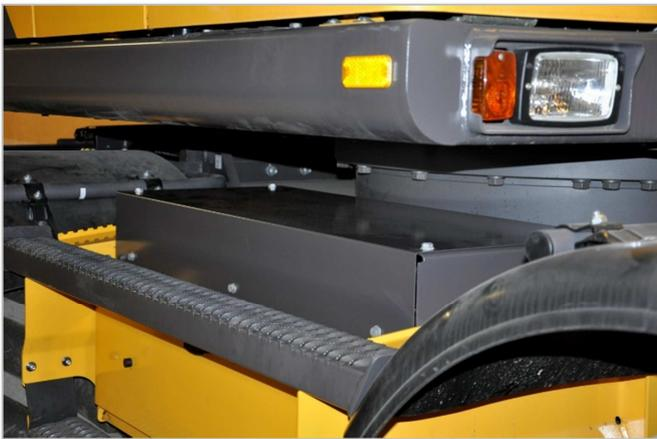
*Cabinet in which the braking system's valves are located.*
