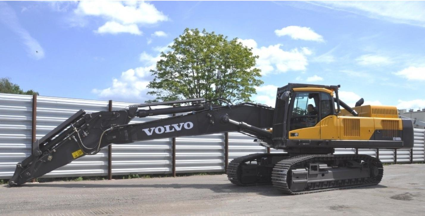
Volvo EC480DL Demolition completed with CeDe Straight boom and protection for arm cylinder.
