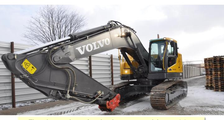
The robust undercarriage has been narrowed down to 3.0 m for an easier transportation in Central Europe
