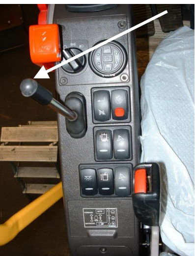
Push button in joystick top for exchanging lifting or tilting operation
