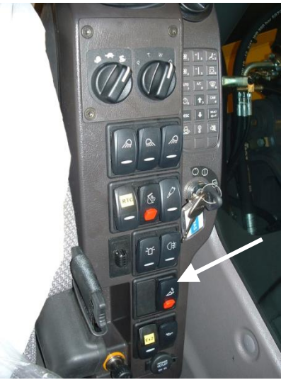
Swicher for disengaging tool locking.
